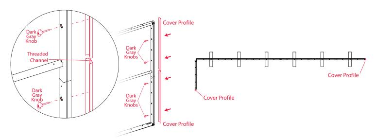
9. To cover the slots at the end of the frames, attach cover profiles with dark gray knobs as seen above. The knobs attach to the cover profile's threaded channel.
