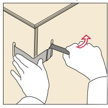
To remove clips, insert the removal tool into the raised pocket on the long leg of clip. Cover the clip with your hand and rotate the tool toward the center of the panel.
