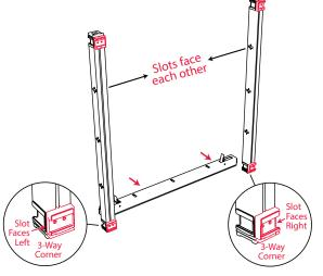
1. Locate two short vertical bars with 3-way corners on both ends. Attach the two together with a horizontal bar by lifting the lock levers and sliding the parts together.
