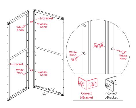
6. Connect the two frames together witht two standard L-brackets and four white knobs. This forms the back/left corner of the display.
