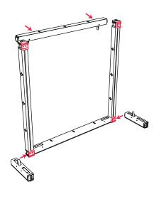
2. Attach two short horizontals to the bottom 3-way corners. Attach a long horizontal to the top of the verticals. Do not lock levers on the small horizontals until step 3.
